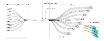
The connection between the blade and module is made with fiber optic assemblies. Utilizing pre-engineered staggers, the assemblies dress perfectly into the blade.
